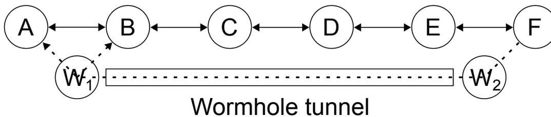
**Figure 2.2.:** Schematics of a wormhole attack. Nodes  $\textcircled{A}$  to  $\textcircled{F}$  are legitimate nodes,  $\textcircled{W}_1$  and  $\textcircled{W}_2$  wormhole endpoints. The dashed line indicates the path of a frame captured and forwarded through the wormhole tunnel by node  $\textcircled{W}_2$  and then being retransmitted by  $\textcircled{W}_1$ .
