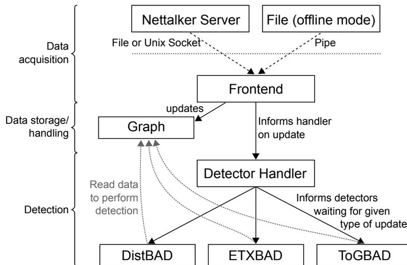
**Figure 7.1.:** This figure gives an overview on the layout of the ToGBAD implementation. Data acquisition relies on external programmes, i.e. the NTS or being fed through a pipe and uses the acquired data to update a graph object. The object will then be read by the detectors to allow them performing their detection process.
