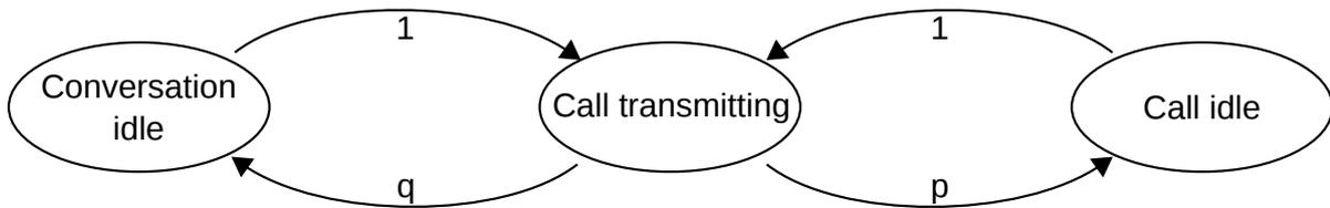
**Figure 5.4.:** The three state semi-Markov model for radio conversations proposed in [8].
