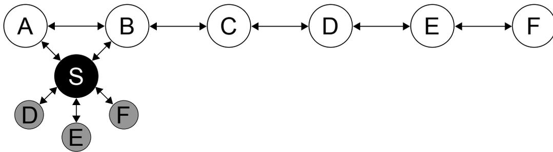
**Figure 2.1.:** Schematics of a sinkhole attack in OLSR. Nodes  $\textcircled{A}$  to  $\textcircled{F}$  are legitimate nodes,  $\textcircled{S}$  is perpetrating a sinkhole attack by claiming to be a neighbour of nodes  $\textcircled{D}$  through  $\textcircled{F}$  (shaded nodes) while it is in fact only a neighbour to nodes  $\textcircled{A}$  and  $\textcircled{B}$ .
