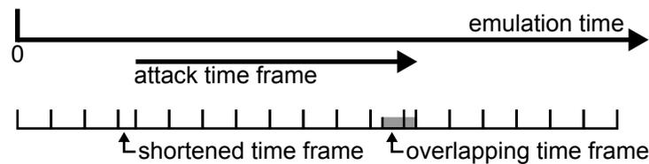
**Figure 7.2.:** For determining false positive/negative ratios, the emulation time will be divided in time frames, indicated by small brackets below the bar representing the emulation time. Time frames will be shortened when an attack starts within them or moved to align their end with an attack's end, if it would otherwise occur within the given frame.
